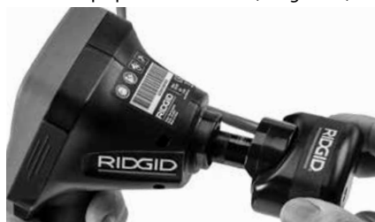
Figur 18 – Kameraets tilkopplingsplugg installert
