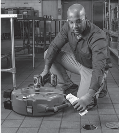
Figure 13 – Applying Lubricant to the Cable Sheath
